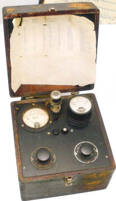
The early device seen above regulated the voltage and the timing for X-ray exposures of different parts of the body, as noted on the chart pasted to its lid.
